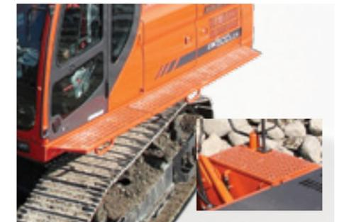
**Cat walk (platform) as standard on DX480LCA & DX500LCA**
